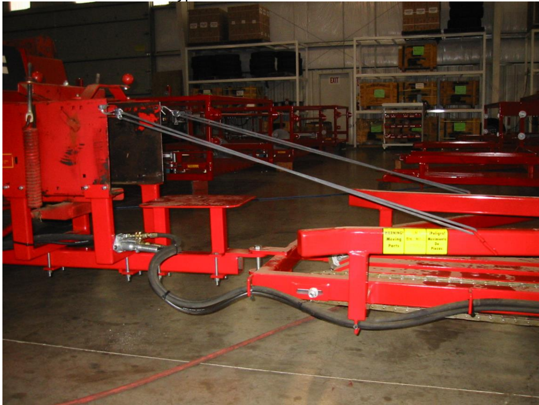
Typical Baler Hitch Installation
